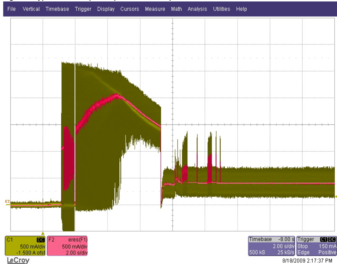
Figure 2. Typical 12V startup and operation current profile
